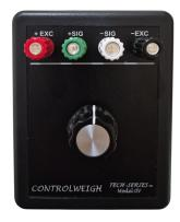
Totalcomp Transducer simulator (TS-0V) are used to test digital weight indicators in weighing equipment. The indicator can be precalibrated prior to installing the load cells and using test weights to calibrate the scale. A indicator with set points can be tested to determine the accuracy.
